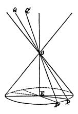
is the vertex, and the constant angle POE is the semi-vertical angle of the cone.
